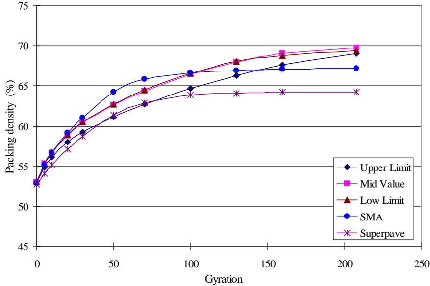
Figure 5: Compaction Curves (Aggregates bigger than 2.36mm)
