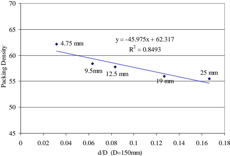
Figure 2: Packing Density with Respect to Relative Scale
