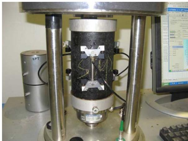
Figure 3: dynamic modulus test of asphalt mastic
