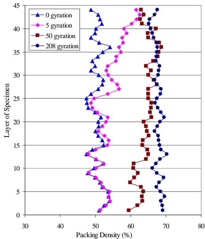
Figure 6: Packing Densities along Specimen Layers
