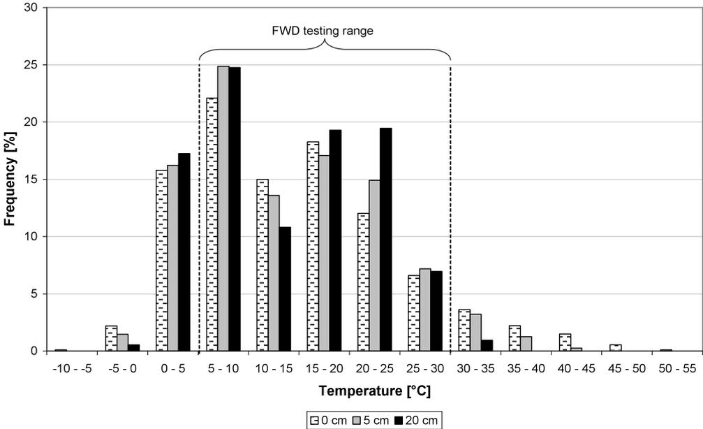
Figure 5: Measured AC temperature distributions at Station 1
