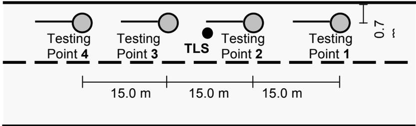
Figure 4: Test setup for repeated FWD testing next to TLS
