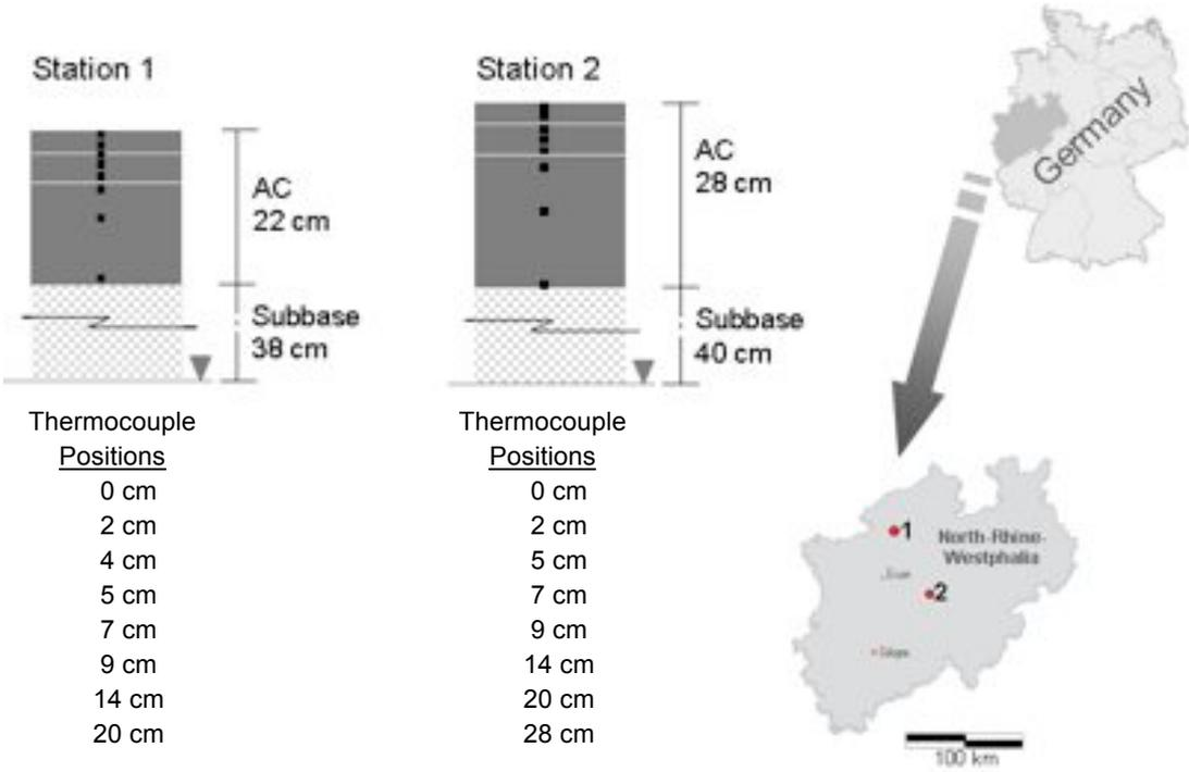
Figure 2: Test site location and inventory data of the Temperature-Logging-Stations (TLS)
