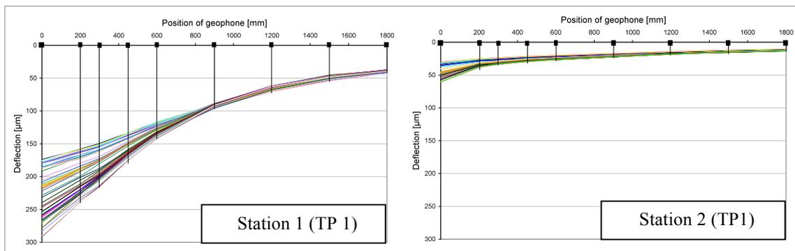
Figure 9: Deflection bowls measured at Station 1 and Station 2 (5 to 35 °C at 5 cm depth)
