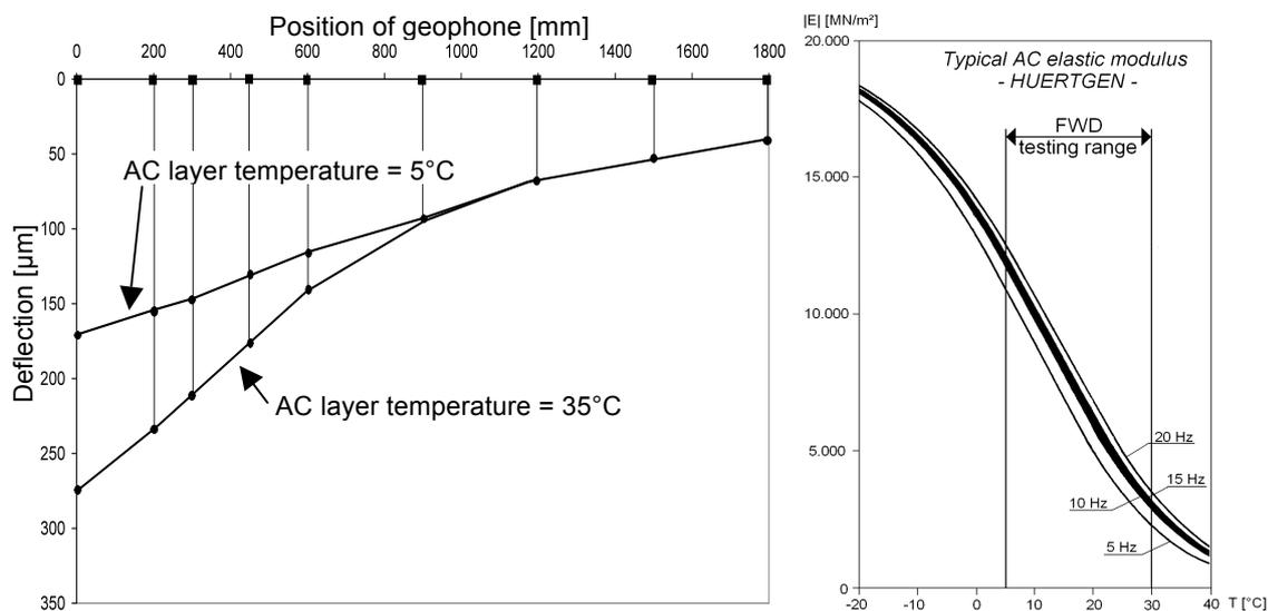
Figure 1: Influence of AC layer temperature on FWD deflection basin and calculated AC elastic modulus
