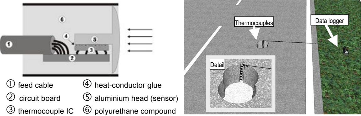
Figure 3: Thermocouple and TLS
