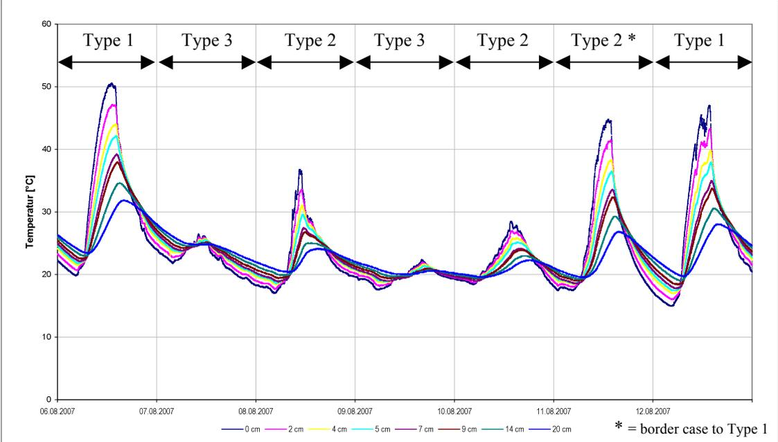
Figure 8: Example of AC surface temperature types
