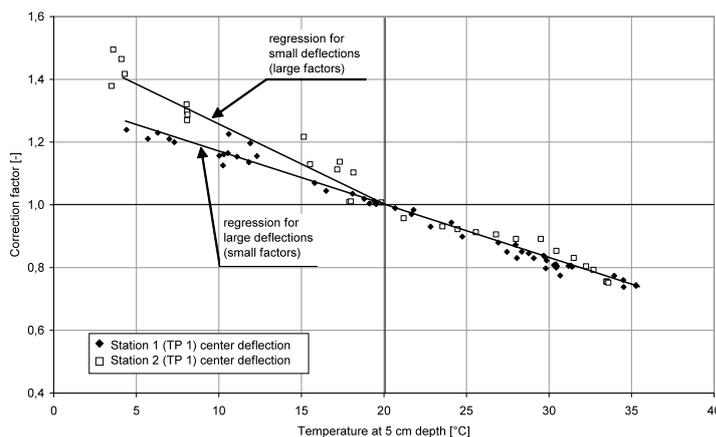
Figure 11: Correction factors (Station 1 (TP 1) and Station 2 (TP 1)) with regression lines
