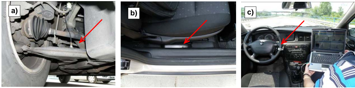
Figure 5: Positions of accelerometers: a) on the wheel holder, b) on the chassis, c) on the steering wheel
