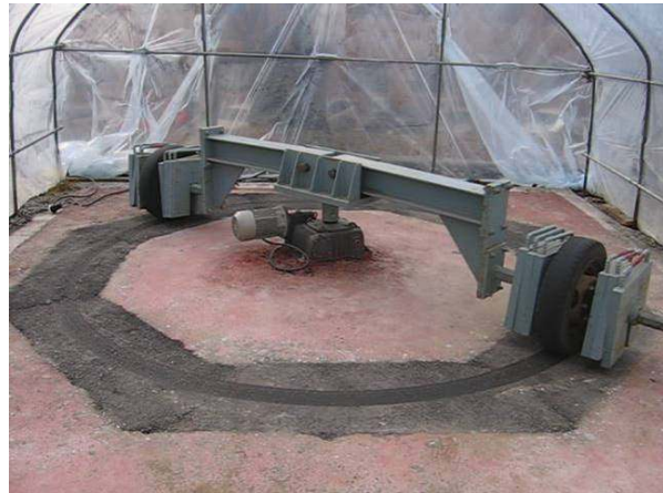
Figure 5. Field-simulated circular wheel tracker
