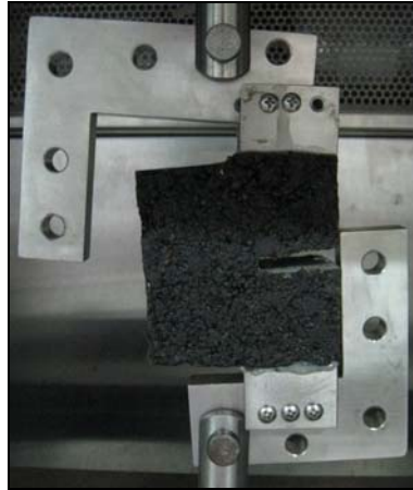
Figure 3: Deformed specimen and misaligned fixture on initial Arcan configuration.
