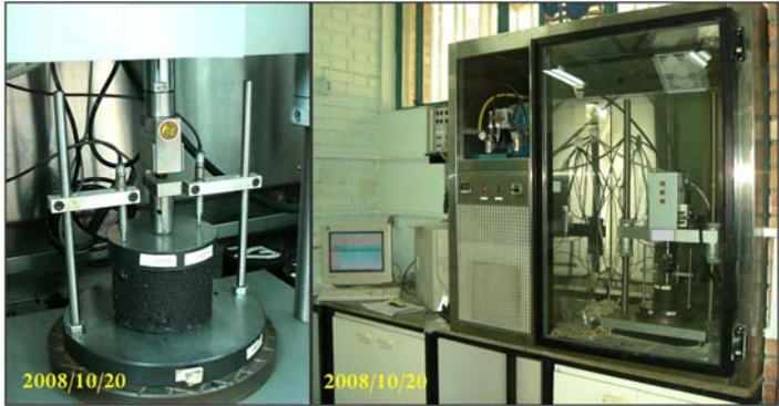
Figure5: UTM (right) and specimen mounted in the machine for dynamic creep test (left).
