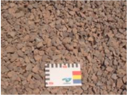
Photo 8: Reclaimed Brick Aggregates (5-13 mm)
