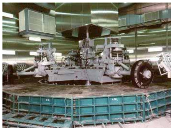
Photo 3: Accelerated Loading and Environmental Simulator (ALES)
