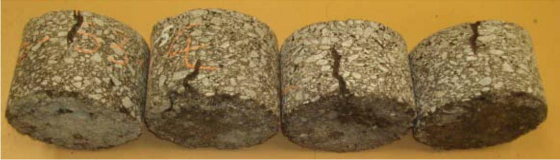
Figure 3: Top-down and bottom-up fatigue cracks in aged test sections (Lane 5 CR-TB).
