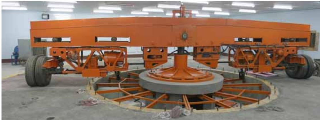
Figure 1: Circular track loading facility (CCRDI)
