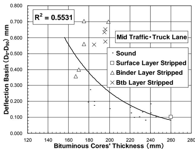
Figure 4: Deflection basin  $D_0-D_{900}$  (corrected at 20°C) and bituminous cores' thickness for porous asphalt having granular subbase layer
