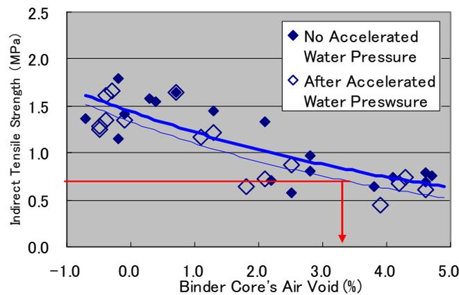
Figure 7: Indirect tensile strength of binder mix and its air voids, sampled from porous asphalt having granular subbase layer
