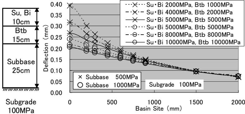
Figure 2: Deflection curves using GAMES in simulation of FWD measurements
