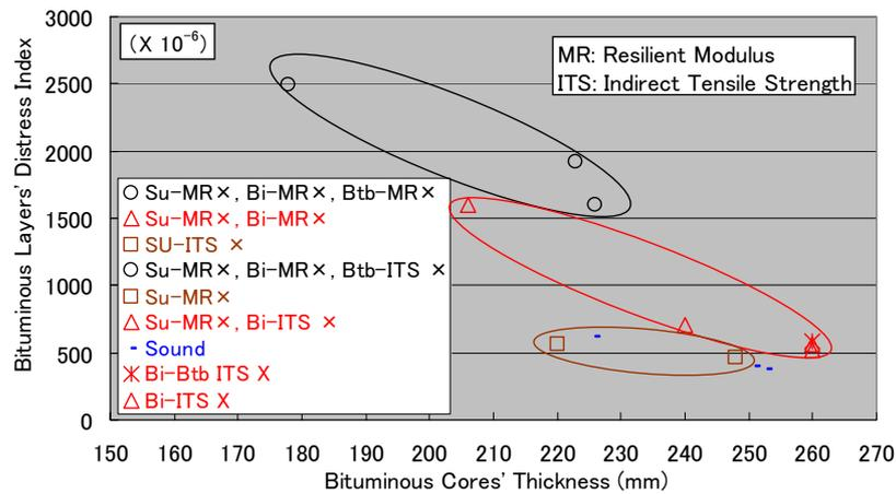
Figure 6: Bituminous layers’ distress index and conditions of resilient modulus and indirect tensile strength for porous asphalt having granular subbase layer
