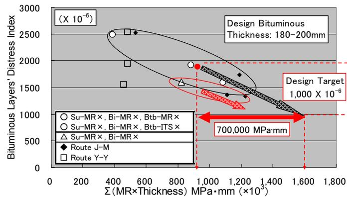
Figure 8: Distress index and summation (core's MR x thickness)
