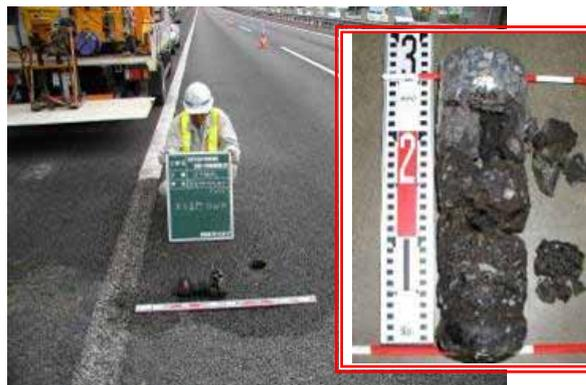
Photo 2: Sampled core from porous asphalt just before rehabilitation
