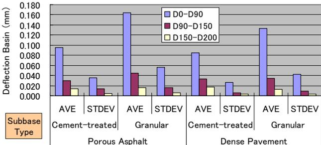
Figure 1: Average and standard deviation of deflection basin data (10,000 measurements)
