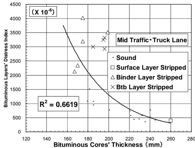
Figure 5: Structural distress index ( $D_0-D_{900}$  / cores thickness) and bituminous cores' thickness for porous asphalt having granular subbase layer
