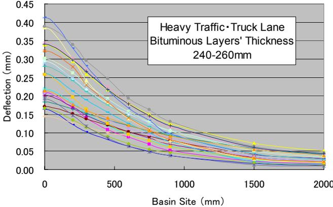
Figure 3: Deflection curves (corrected at 20°C) from a real motorway section with porous asphalt having granular subbase layer
