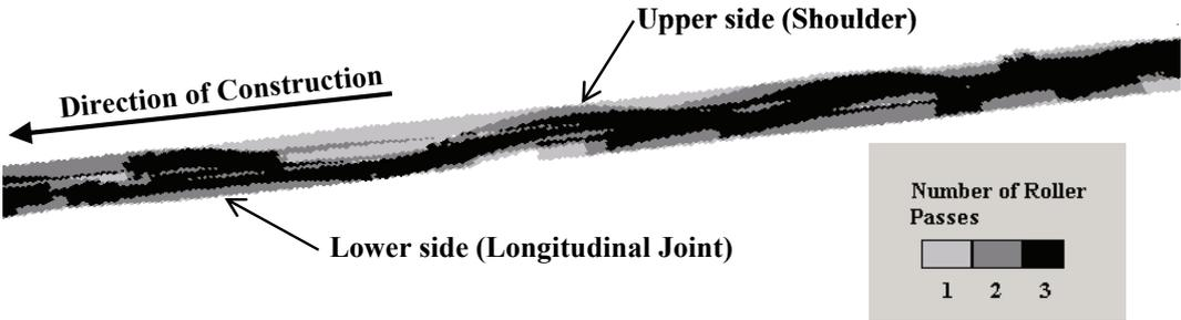
Figure 1: Inconsistent roller passes over the pavement (Scherocman et al., 2006)
