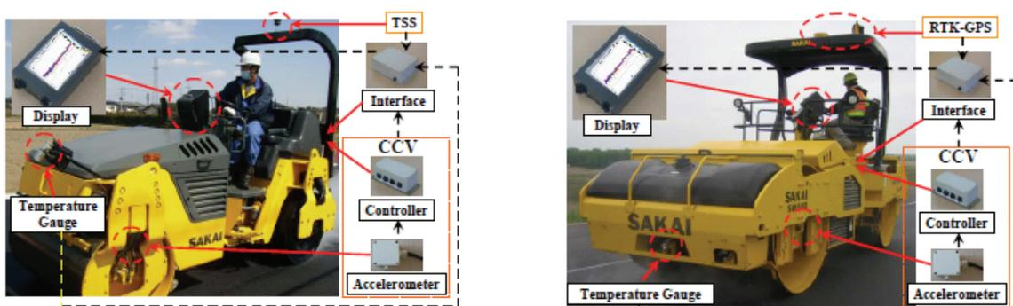
Figure 2: Sakai IC systems used in Japan (left) and the USA (right)
