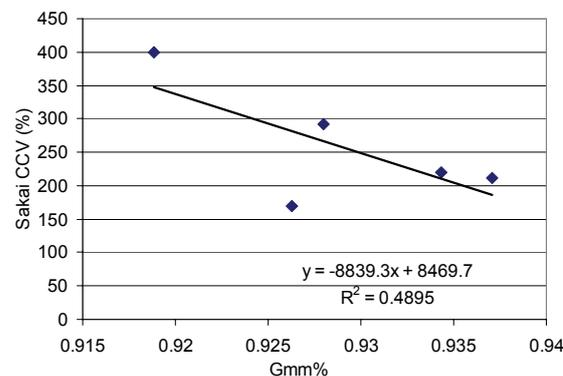
Figure 6: Inverse correlation of HMA core densities vs. CCV
