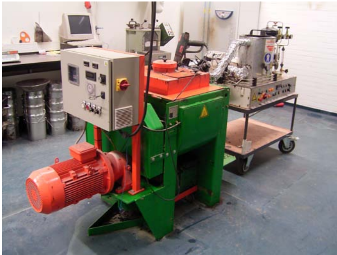
Figure 1: Lab mixer and foam unit to prepare a half warm mix in the lab
