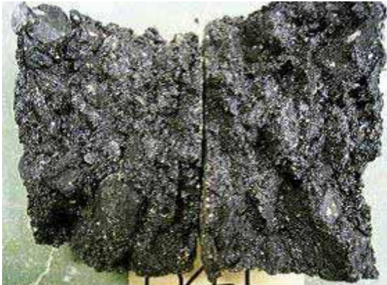
Photo 3: Conditioned specimen after Marshall Stability Test
