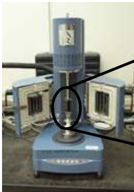
(e) Testing FAM specimens using the DMA
