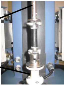
(e) Testing FAM specimens using the DMA
