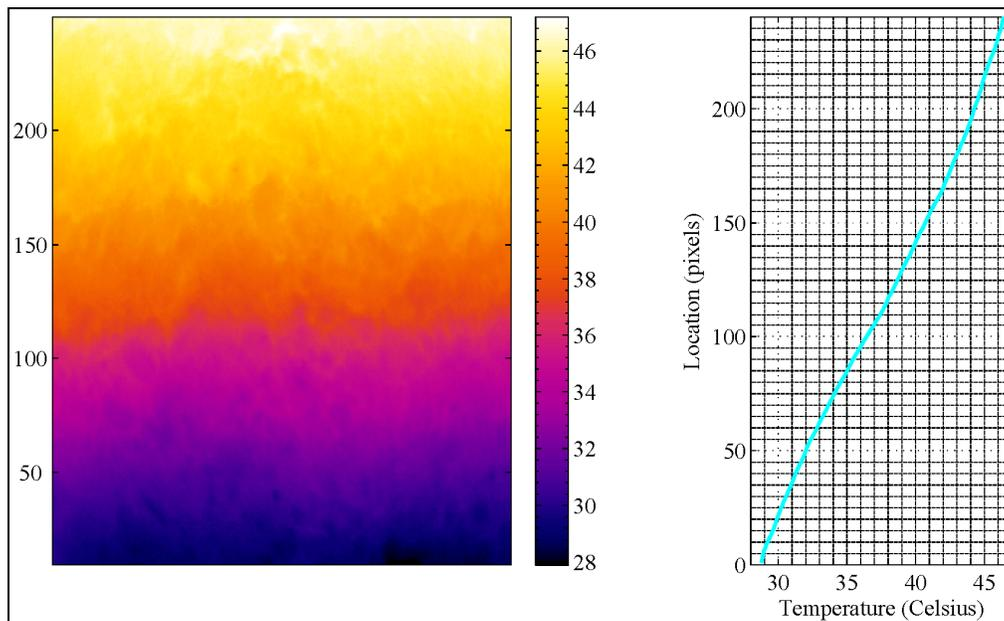
Figure 3: Heat Transfer Across Newly Constructed Warm Mix Asphalt Joint
