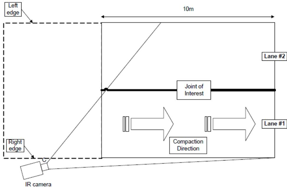
Figure 1: Infrared Video Collection Arrangement
