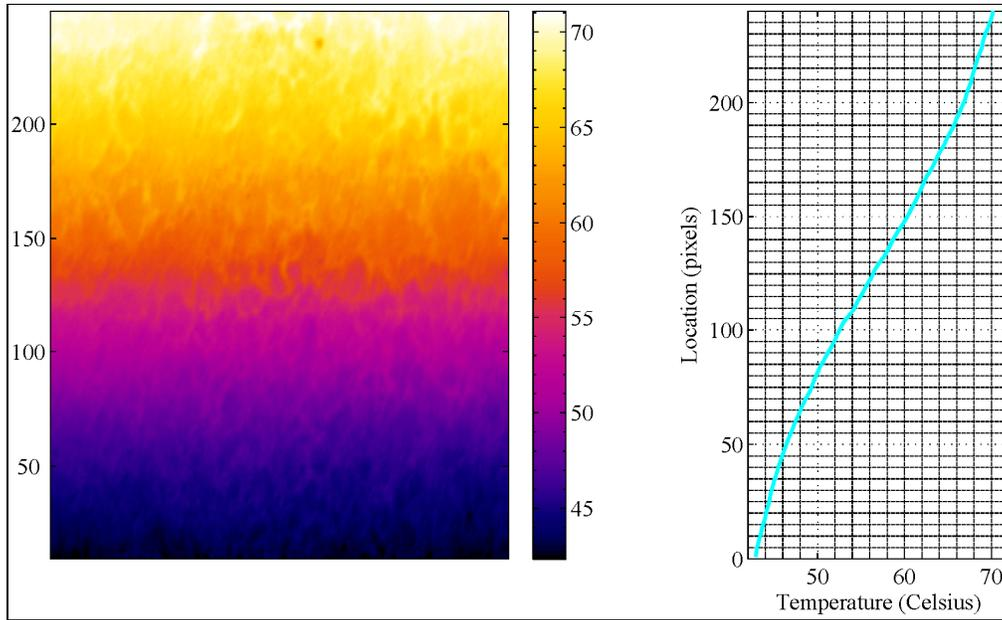
Figure 5: Heat Transfer Across Newly Constructed Hot Mix Asphalt Joint
