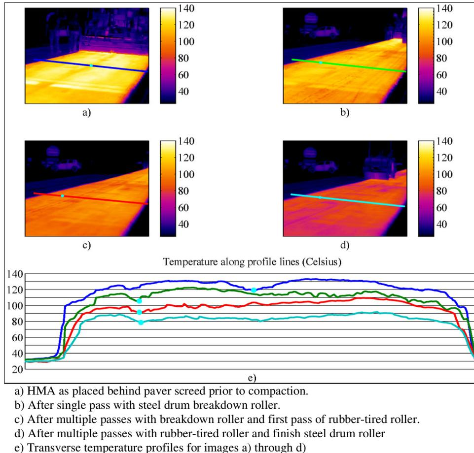
Figure 4: Thermal Video and Profiles of Hot Mix Asphalt Section on Victoria Road
