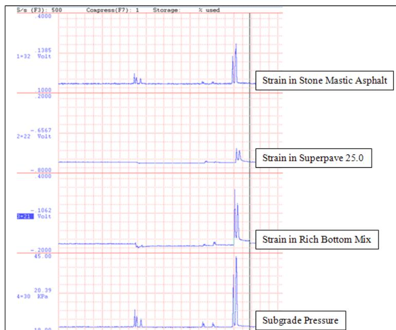
Figure 3: Example of Strains and Pressure Recorded for a Passage of a Three Axle Truck. Note: the vertical volt scale (representing strain) is different at each location.
