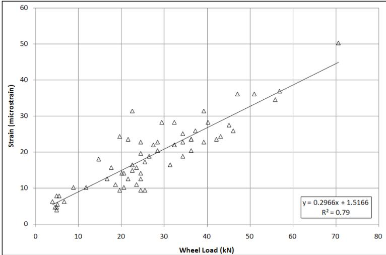
Figure 4: Relationship of Wheel Load versus Tensile Strain in RBM determined on July 2, 2009.
