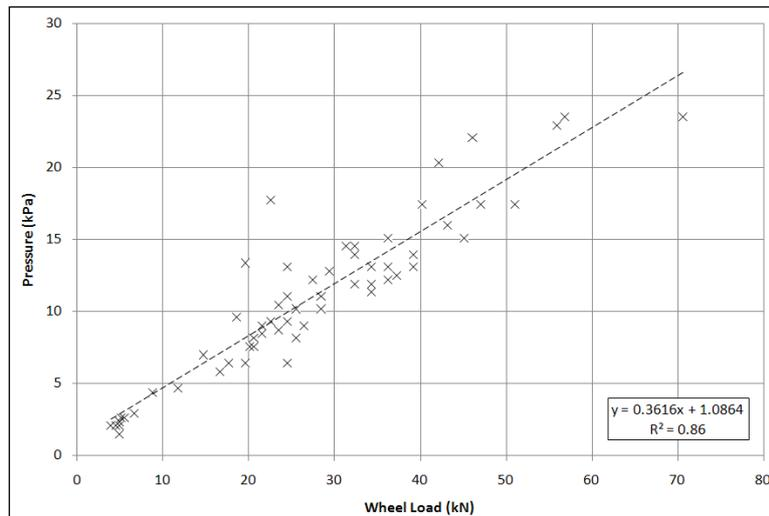
Figure 5: Wheel Load versus Subgrade Pressure determined on July 2, 2009
