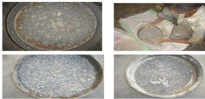
Photo 2: Sieve Analysis to find out Fibres in Dry Aggregate
