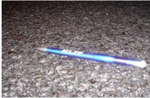
Photo 11: Final Texture of Newly Laid Surface of SMA
