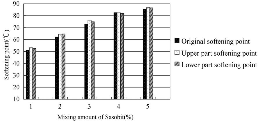
Figure 2: Softening points of modified asphalts with different mixing amount of Sasobit before and after segregation tests.
