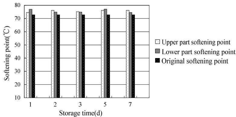
Figure 4: Softening points of modified asphalts with different storage time before and after segregation tests.
