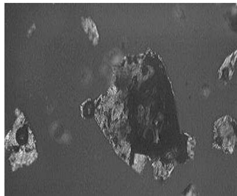
Figure 9: The metallograph of Sasobit wax.
