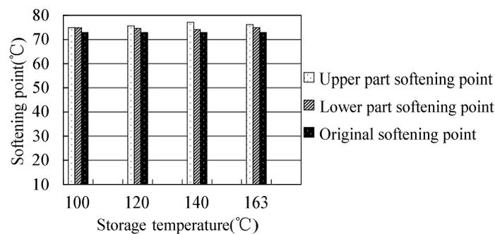
Figure 6: Softening points of modified asphalts with different storage temperature before and after segregation tests.
