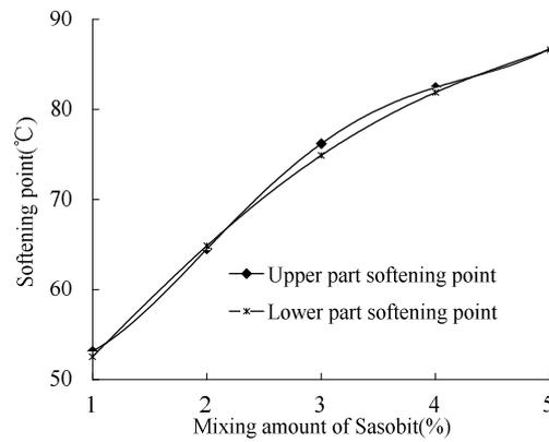
Figure 3: Influence on the storage stability of modified asphalt under different mixing amount of Sasobit.
