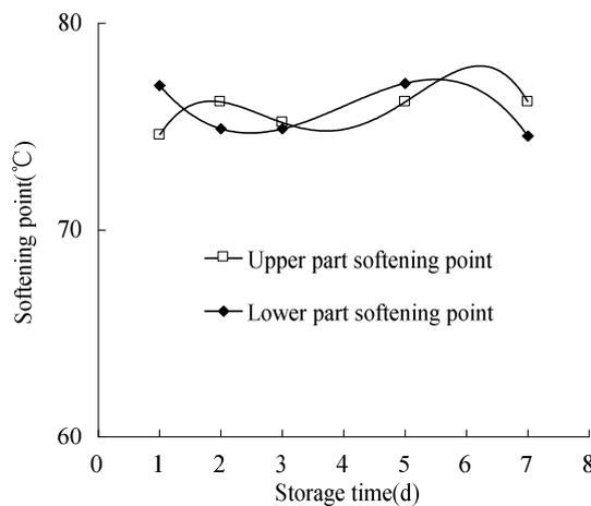
Figure 5: Influence on the storage stability of modified asphalt under different storage time.
