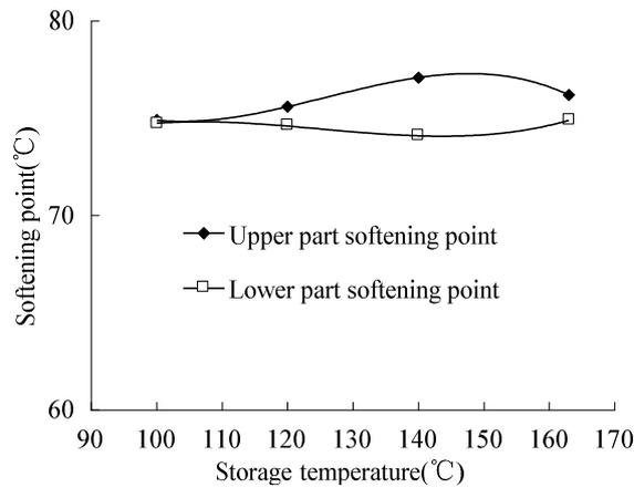
Figure 7: Influence on the storage stability of modified asphalt under different storage temperature.
